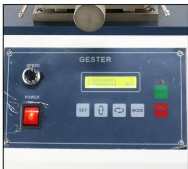
COUNTER: set and record the test times.
